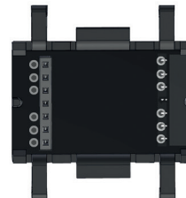
Fig.: Input bus connector for the 800-CON-RJ45 transfer module at the input of a series of measurement devices and modules.
